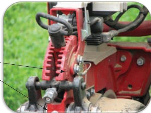
**Equipment Solution:** White planters come standard with the most accurate depth control system in the industry. Rows may be calibrated prior to the season so that depth is accurate and known for all rows.
